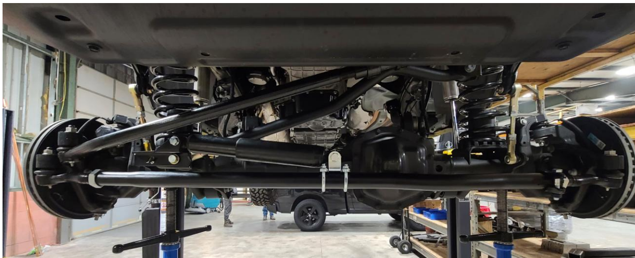
Figure 1: Front axle supported with two adjustable jack stands and tires removed
