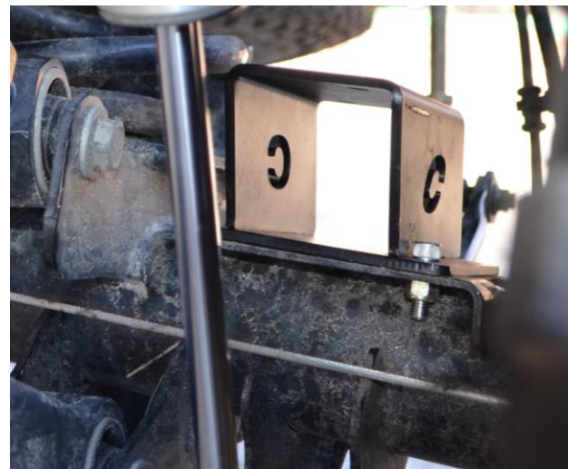
Figure 31: Bump-stops (1" tall and 3" tall bump-stop options)
