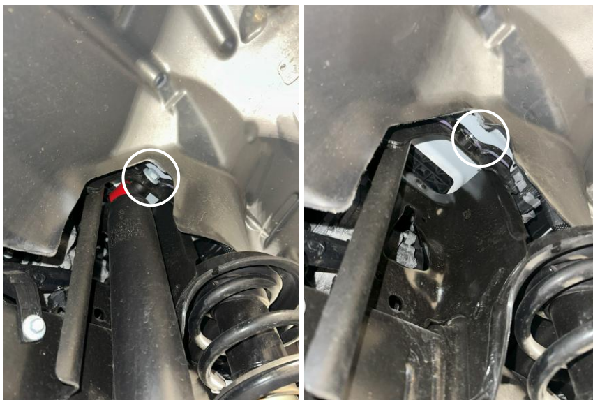
Figure 5: Front upper passenger shock bolt removed
