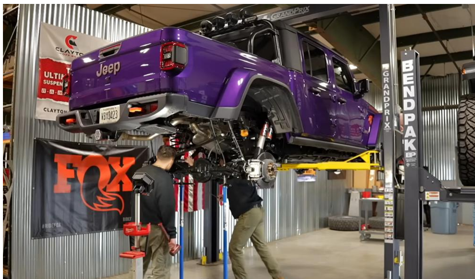
Figure 19: Rear tires removed, axle drooped
