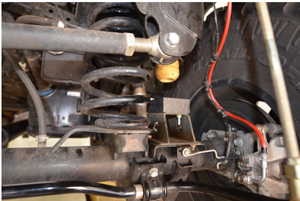
Figure 37: Rear Gladiator Extended Brake Lines installed
