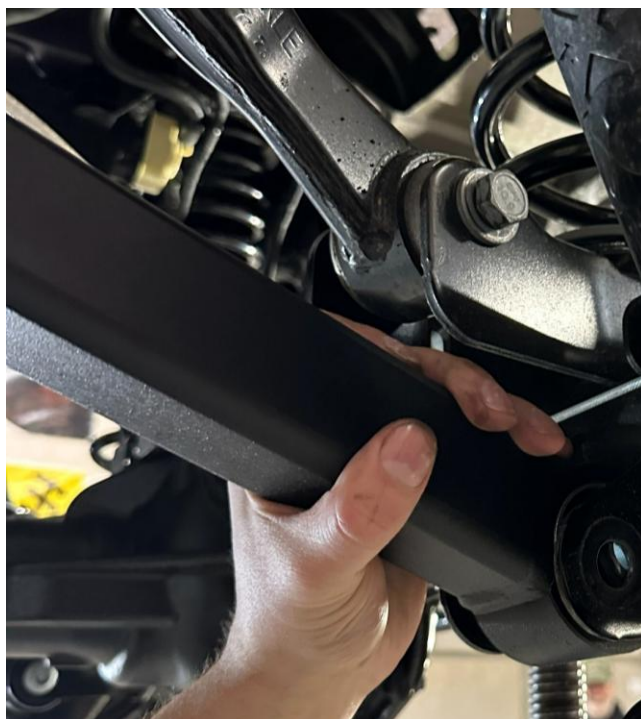
Figure 27: New driver-side control arms installed with original hardware
