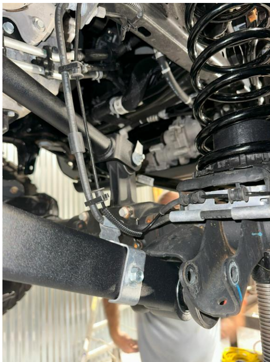
Figure 15: Brake line brackets secured (Brake line extension bracket on far right, only supplied in 3.5"+ kits)
