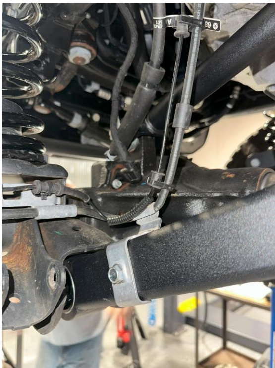
Figure 15: Brake line brackets secured (Brake line extension bracket on far right, only supplied in 3.5"+ kits)
