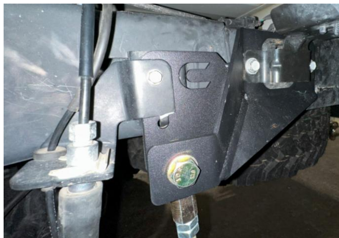
Figure 4: Installed bracket (driver side)
