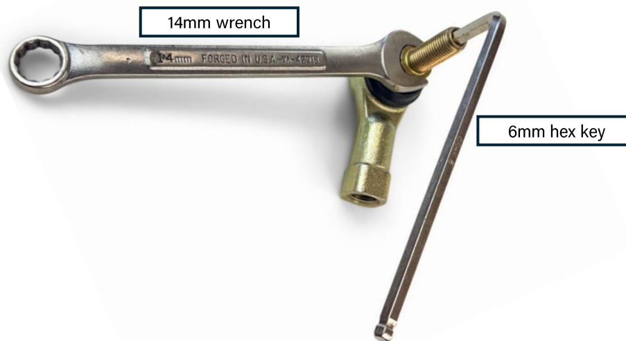
Figure 5: Rod end tightening options
