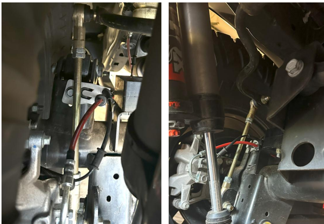
Figure 7: Correct sway bar angle
