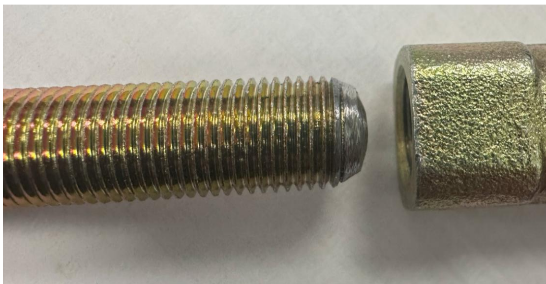
Figure 4: Beveled edge of sway bar rod with sway bar rod end
