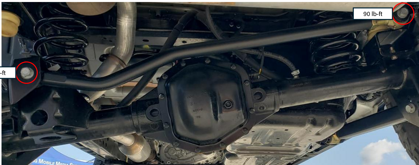
JL adjustable track bar installed with proper orientation and torque
