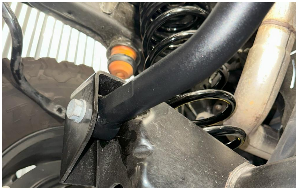
JL adjustable rear track bar bolt installed hand-tight (axle-end)
