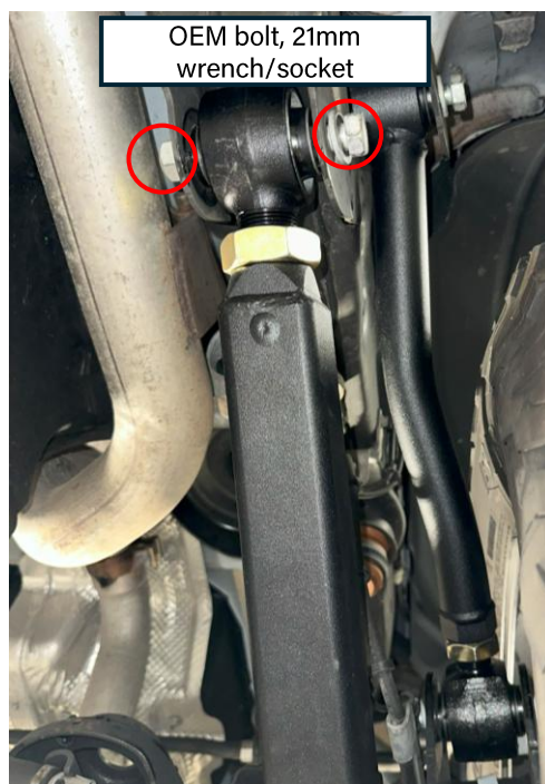
1709102 (OVERLAND+ Series) Rear lower control arm installed (frame-end and axle-end)
