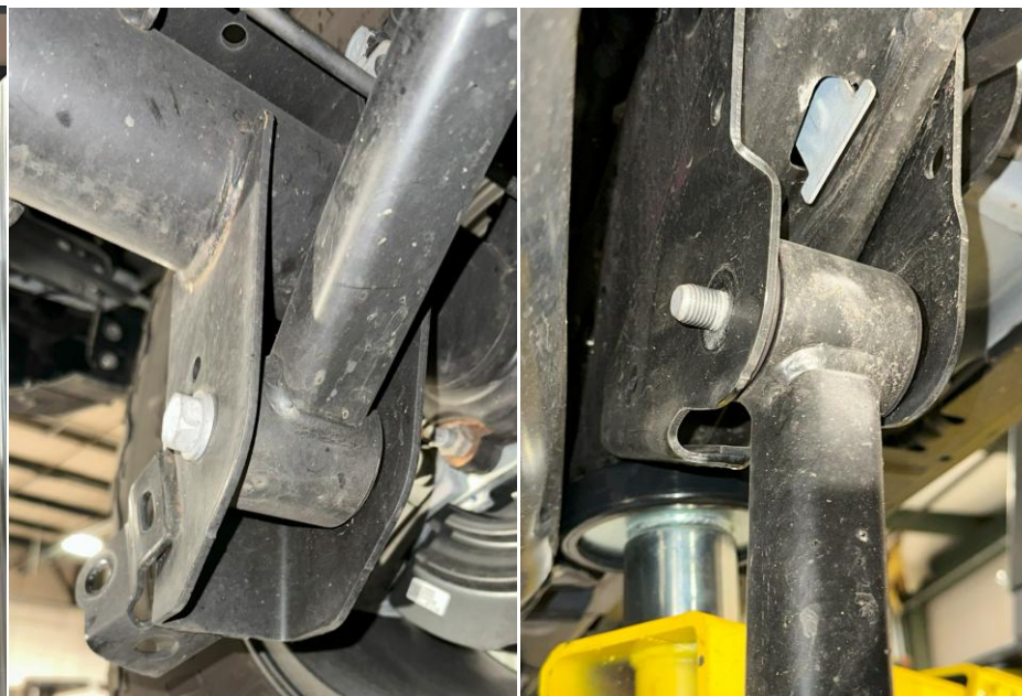
Jeep JL rear lower control arm mounts (axle and frame)
