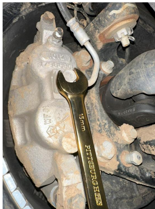
Brake caliper banjo bolt (15mm)
