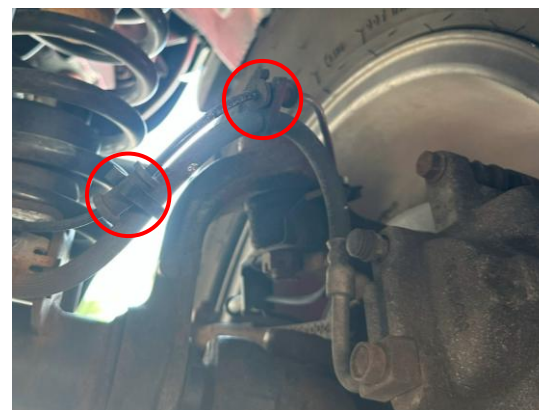
Old brake-line clips to be removed
